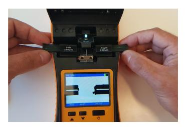
Other manufacturers may say that You should use tops/cloth and alcohol to clean a V-groove but that is not working well. There's a big risk that You contaminate the V-groove even more with small fabric-parts from the tops/cloth.
